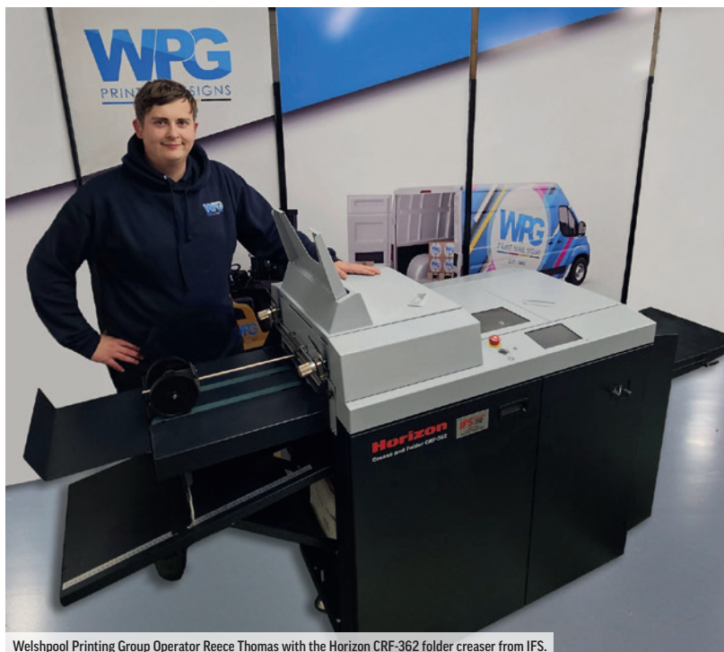
Welshpool Printing Group Operator Reece Thomas with the Horizon CRF-362 folder creaser from IFS.
