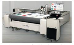
enables users to work with stocks up to 25mm in thickness such as Dibond, MDF and acrylic.
