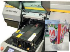
Mimaki Europe launched their brand new Kebab HS, debuting worldwide at FESPA. Serving as an optional system for Mimaki's renowned UJF Series flatbed UV printers, the Kebab HS enables seamless 360 degree printing on cylindrical objects, such as bottles and tumblers. This latest solution can also print directly on tapered objects, including glasses and cups.
