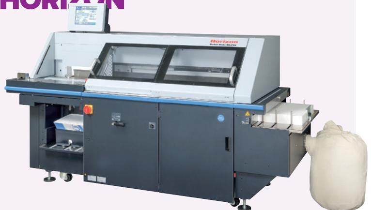
It includes an automated, sensor-activated digital caliper system which consistently measures book block thickness and automatically transfers this data to the binder for quick, automated set-up for books of different thicknesses. It features a large 10.4" intelligent colour touch-screen, job programming, and a compact configuration.
